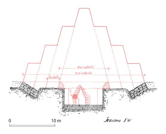
**Fig. 9.** Reconstructed section of the satellite pyramid of Meidum according to Maragioglio and Rinaldi ((1964), tav. 7 (fig. 3)). The reconstructed part is shown in red. The blocks at the base of the central core are hypothetical.
