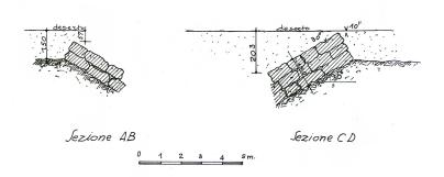
Fig. 7. Cross-section of the blocks on the edge of the satellite pyramid of Meidum (after Maragioglio and Rinaldi (1964), tav. 7 (fig. 4)).
