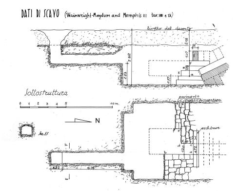
Fig. 6. Cross-section and plan view of the satellite pyramid of Meidum (after Maragioglio and Rinaldi (1964), tav. 7 (fig. 1)).
