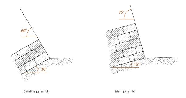
Fig. 10. Construction techniques with sloping layers applied at Meidum.
